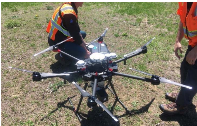
Figure 1. AirShark's UAV drone with LiDAR components attached, prior to takeoff.
